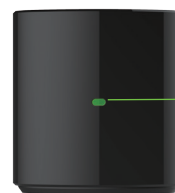
LED Indicator Indicates power and status
