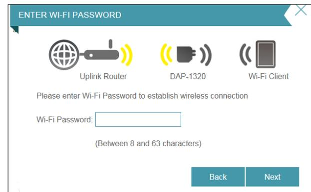
The DAP-1320 will rebroadcast the Wi-Fi connection from the uplink router as an *Extended Network*. Enter an **Extended Wi-Fi network name** and **Extended Wi-Fi network password**.
