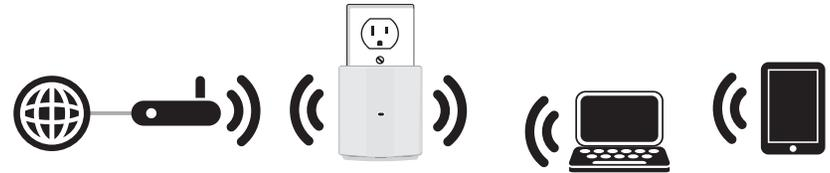
**Step 6** - Next, connect your wireless devices. From your wireless device, go to the Wireless Utility to display the available wireless networks.
