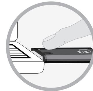
**Step 3** - Allow up to two minutes to connect. Once the connection is successful the LED will be solid green and your wireless connection will be secured with WPA2.
