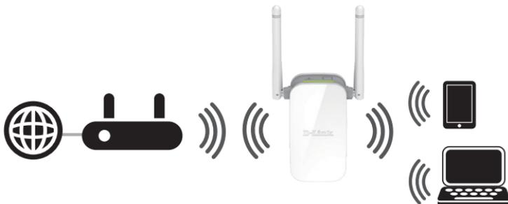
If the signal strength indicators are showing one single amber bar or if the DAP-1325 is not connecting, move the DAP-1325 to a wall outlet closer to your wireless router or access point.
