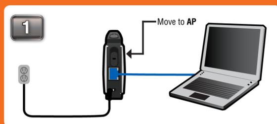
Move the selection switch to **AP** on the back of the DAP-1350. For setup purposes, connect the DAP-1350 to your PC. Follow the steps on the other side of this poster to assign your computer a static IP address.
