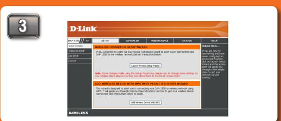
You will then be directed to the device's setup page with two options. Click the "Launch Wireless Setup Wizard" to begin the setup.
