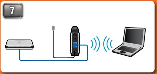
Once the device has been disconnected and your computer's IP address has been restored back to the previous settings, connect the Ethernet cable from the DAP-1350's Ethernet port to your switch or router. Now you are able to connect your laptop wirelessly to the device.
