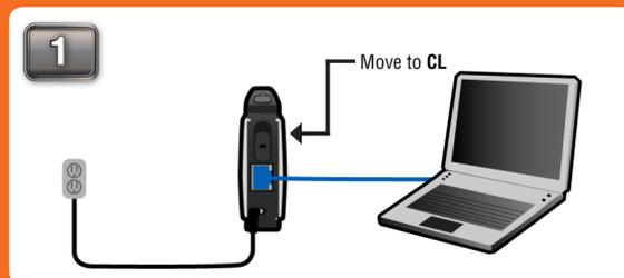
Move the selection switch to **CL** on the back of the DAP-1350. For setup purposes, connect the DAP-1350 to your PC. Follow the steps on the other side of this poster to assign your computer a static IP address.
