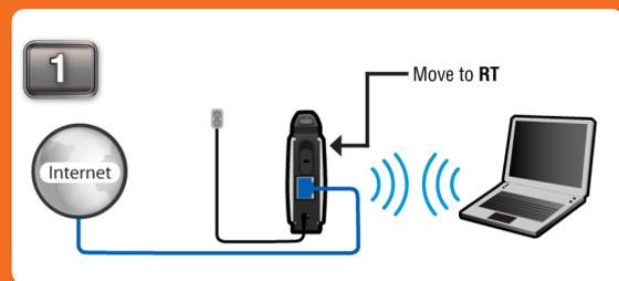
Move the selection switch to **RT** on the back of the DAP-1350. Connect the DAP-1350 to your broadband modem or Internet connection. You must connect wirelessly to configure the pocket router. The default SSID is dlink.
