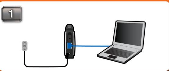
Connect the power cable to the router. Then connect your ethernet cable to the DAP-1350's Ethernet (LAN/WAN) port on the back.
