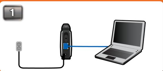
Begin by connecting the power cable to the DAP-1350. Then, connect your ethernet cable to the device's Ethernet (LAN/WAN) port on the back.
