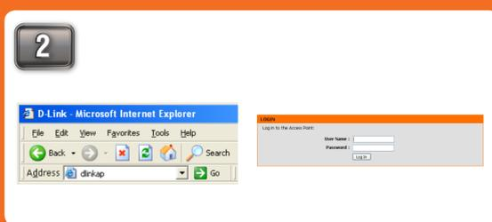
Once connected to the device, open your web browser and type in the address bar "http://192.168.0.50" or "dlinkap" and then press ENTER. Type "admin" and then enter your password. Leave the password blank by default. Click Log In to continue.
