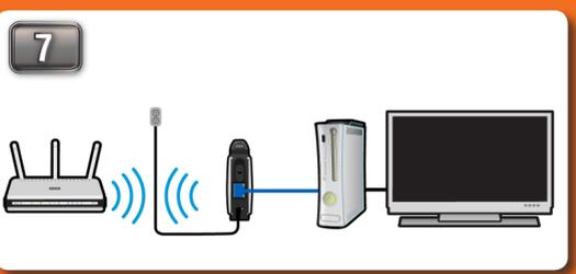
If you are going to connect this to another device like a game console, then disconnect the Ethernet cable from your computer and then connect to the device. Make sure the IP settings on your device are within the same network.
