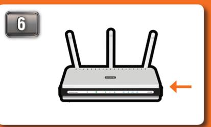
Press the PBC button on your router within 120 seconds. Wait until the WPS LED on the DAP-1350 stops blinking. Refer to your router's manual for more information.
