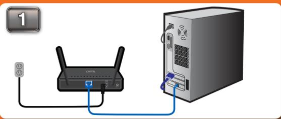
Connect the power cable to the router. Then connect your ethernet cable to the DAP-1360's LAN port on the back.
