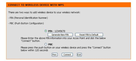
Start WPS on the wireless device you are adding to you wireless network to complete the setup.
