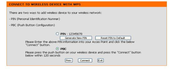
Press down the WPS Button on the wireless device you are adding to your network to complete the setup.
