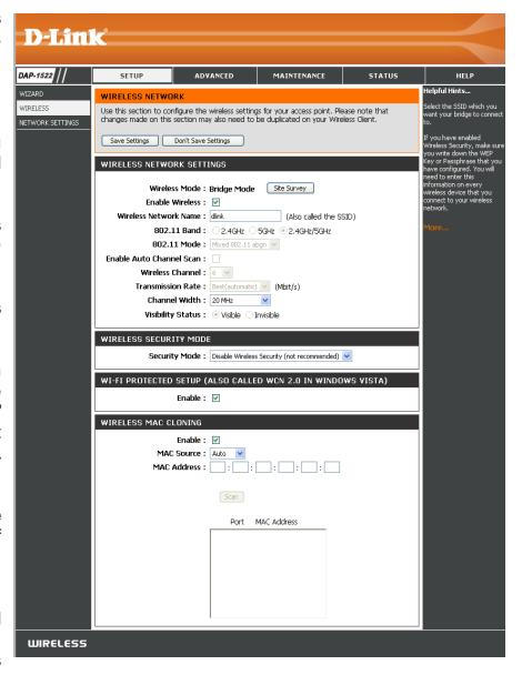
**Transmission** Select the transmit rate. It is strongly suggested to select Best (automatic) for best performance. This option is unavailable Rate: in Bridge Mode.
