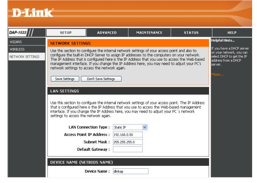
**LAN Connection** Select DHCP to automatically obtain an IP **Type:** address on the LAN/private network.
