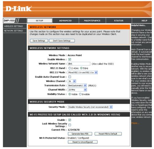
**Enable Auto** The Auto Channel Scan setting can be selected to allow the DAP-1522 to choose the channel with the least amount of **Channel Scan**: interference.
