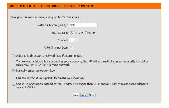
For WPA encryption, enter a Network Key between 8 and 63 characters long or enter exactly 64 characters using 0-9 and A-F.
