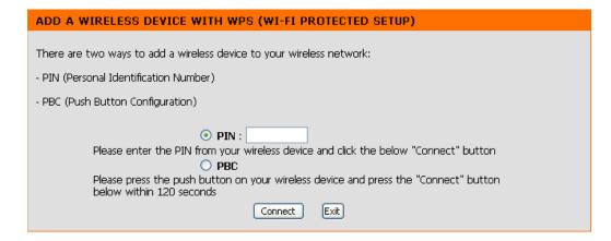
Start **WPS** on the wireless device you are adding to you wireless network to complete the setup.
