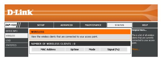
**Signal:** This is a relative measure of signal quality. The value is expressed as a percentage of theoretical best quality. Signal quality can be reduced by distance, by interference from other radio-frequency sources (such as cordless telephones or neighboring wireless networks), and by obstacles between the access point and the wireless device.
