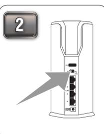
With the DAP-1525 powered off, select the mode you want to use by sliding the selector on the back of the device.
