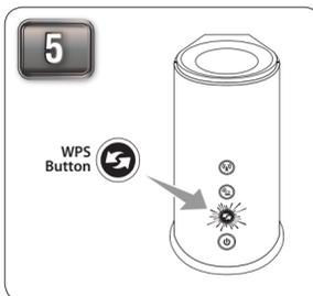
For **One Touch Configuration**, press and hold the WPS button on the DAP-1525 for about 5 seconds. The WPS LED will blink.
