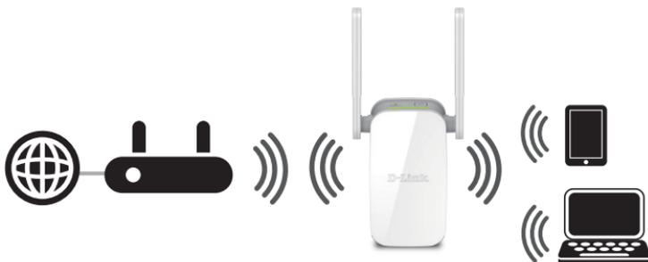
If the signal strength indicators are showing one single amber bar or if the DAP-1610 is not connecting, move the DAP-1610 to a wall outlet closer to your wireless router or access point.
