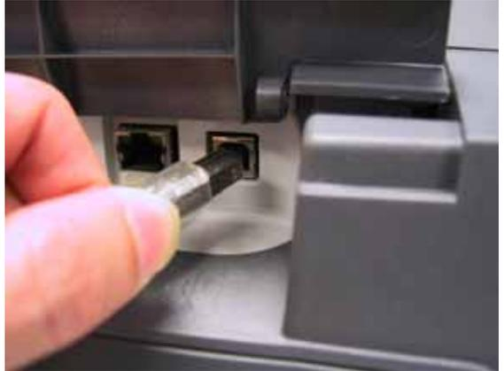
Using the included power adapter, connect the yellow coded plug to the yellow power connector port on the **DBT-320** and the other end of the power connector to an available power strip or outlet.
