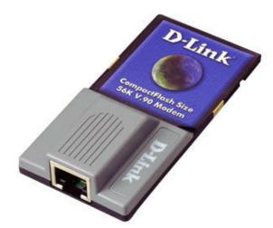
D-Link's DCF-560M is a CompactFlash Modem with an integrated RJ-11 connector, which enables Windows CE-based Palm PC or hand-held devices to connect to the Internet and provide Fax capabilities.
