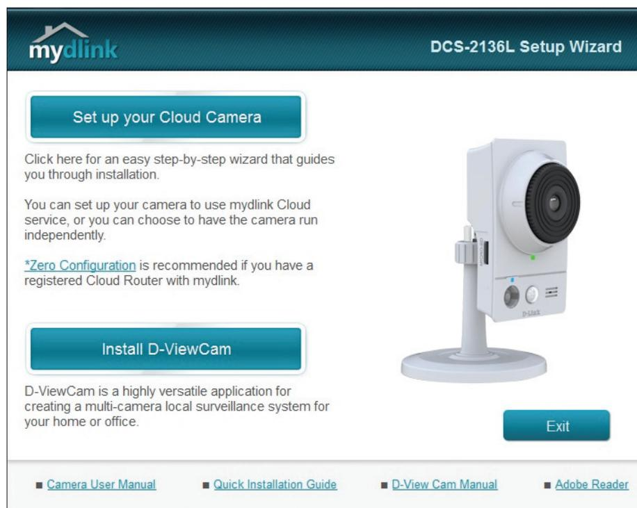
**Note:** At the end of the camera setup process, you will see a summary that includes the camera's IP address. Make a note of it. You will need the IP address for advanced configuration of your camera. Refer to "[Configuration Interface](#)" on page 22.
