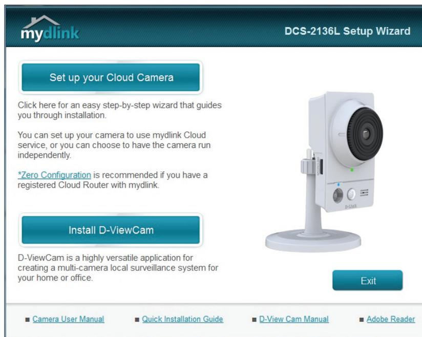
**Note:** At the end of the camera setup process, you will see a summary that includes the camera's IP address. Make a note of it. You will need the IP address for advanced configuration of your camera. Refer to "[Configuration Interface](#)" on page 22.
