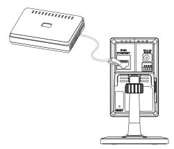
Note: Once power has been established, the LED will turn red. When the device has obtained an IP address and is accessible, the LED will turn green.
