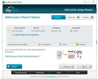
If you wish to remove the camera from a previously registered mydlink account, press and hold the **Reset** button on the rear panel for at least 10 seconds and click **Retry** to restart the *Setup Wizard*.
