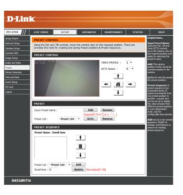
Preset List: To add a preset to the sequence, select it from the dropdown box at the bottom of this window, set the **Dwell time** to determine how long the camera view will stay at that preset, then click the **Add** button. The preset name will appear in the list, followed by the dwell time to view that preset for.
