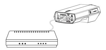
**Note:** Once power has been established, the LED will turn red. When the device has obtained an IP address and is accessible, the LED will turn green.
