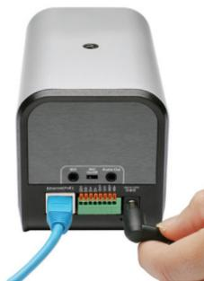
**Note:** When you have a proper connection, the LED on the network camera will turn green. The light may go on and off and your computer may show an intermittent loss of connectivity. This is normal until you have configured your Network Camera.
