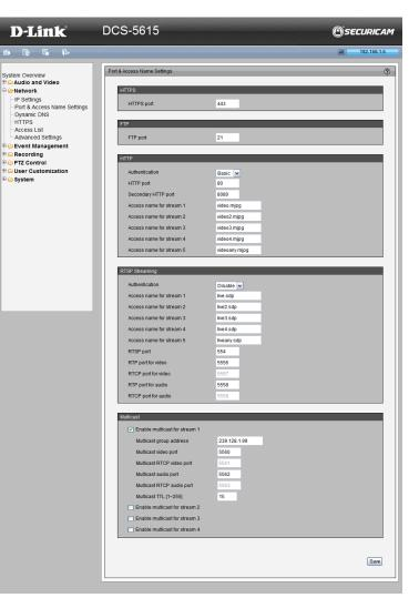
Access name for stream 1 ~ 3: This Network Camera supports multiple streams simultaneously. The access name is used to differentiate the streaming source. When using Firefox to access the Network Camera and the video mode is set to JPEG, users will receive video comprised of continuous JPEG images This technology, known as "server push", allows the Network Camera to feed live pictures to Firefox. And use the following HTTP URL command to request transmission of the streaming data.
