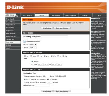
Size of each file for recording: If this is selected, files will be separated based on the file
