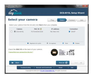
If you wish to remove the camera from a previously registered mydlink account, press and hold the reset button on the rear panel for at least 10 seconds and click **Restart** to restart the wizard.
