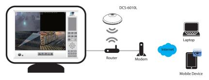
Network Video Recorders (NVRs) are standalone storage devices with a powerful embedded system that can record video from up to 9 network cameras located on local or remote sites into a dedicated HDD storage without turning on a PC. Video and camera management can be done as needed using any computer attached to the network.
