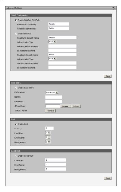
The 802.1x standard is designed to enhance the security of local area networks, which provides authentication to network devices (clients) attached to a network port (wired or wireless). If all certificates between client and server are verified, a point-to-point connection will be enabled. If authentication fails, access on that port will be prohibited. 802.1x utilizes an existing protocol, the Extensible Authentication Protocol (EAP), to facilitate communication.
