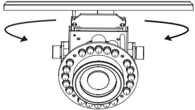
Loosen the tilt screws on both sides of the camera, and turn the lens module up and down until the desired position is achieved; tighten the tilt screws once completed.
