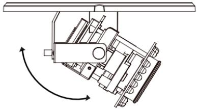
Turn the lens to adjust the IP camera's image until the desired orientation is achieved, tighten the image adjustment screw once completed.
