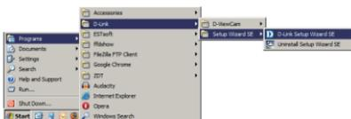
The Setup Wizard will appear and display the MAC address and IP address of your camera(s). If you have a DHCP server on your network, a valid IP Address will be displayed. If your network does not use a DHCP server, the network camera's default static IP **192.168.0.20** will be displayed.
