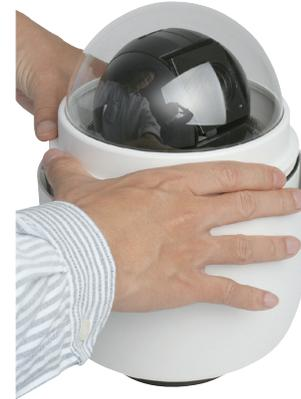
**Warning:** DO NOT press down on the cover, as shown in the figure; this might cause damage to the camera.
