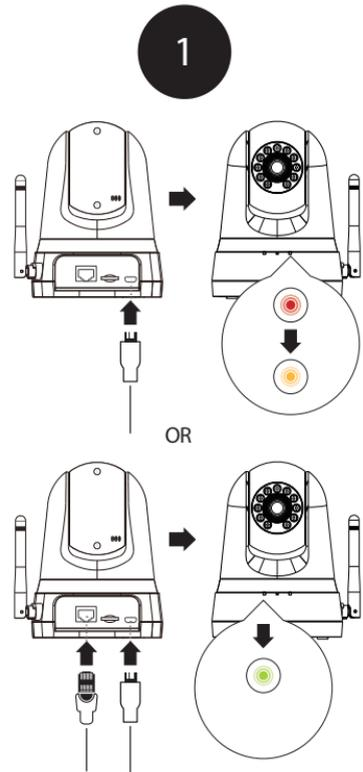
**Wireless set-up:** Plug the included USB Power Adapter into the back of the camera. Wait until the PWR LED changes from red to blinking orange.
