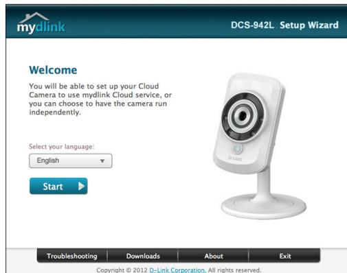
Within 20-30 seconds, the Setup Wizard will open, which will guide you step-by-step through the installation process, from connecting your hardware to configuring your camera and registering it with your mydlink account.
