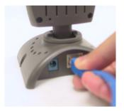
The LAN LED will light green when there is a good connection to the LAN. The LED will begin to flash indicating the camera is receiving or sending data.
