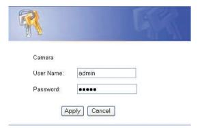
After you successfully log in, the camera will be displayed in your Web browser. In this example the IP address of the camera is <a href="http://192.168.0.20">http://192.168.0.20</a>. Your DCS-950G may have a different IP Address.
