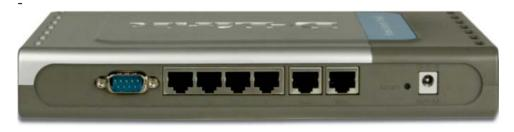
**COM Port:** Serial Read-Only access to the firewall software from a PC equipped with a Serial COM port (9600 baud, 8 data bits, No Parity, 1Stop bit, No Flow Control).
