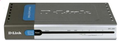
**Power:** A solid light indicates a proper connection to the power supply.
