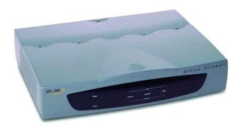
The D-Link DFL-300 Office Firewall is a hardware-based firewall designed for the small office environment.
