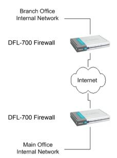
DMZ networks. The networks at the ends of the VPN tunnel are selected when you configure the VPN policy.
