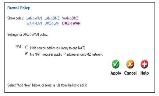
By default the DFL-700 is enabled to perform NAT on both LAN and DMZ interfaces. Disable NAT on the DMZ interface.
