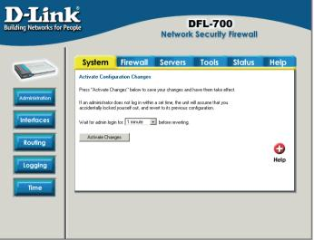
administrator must login again. This has to be done before a configurable timeout has been reached, otherwise the DFL-700 will revert to the previous configuration. The timeout can be set on the Activate Configuration Changes page, by choosing the time from the dropdown menu.
