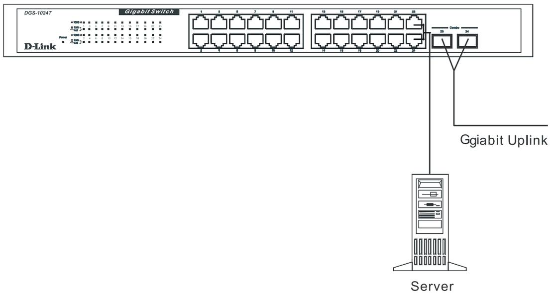
Figure 2- 6. Gigabit connection using optional module port
