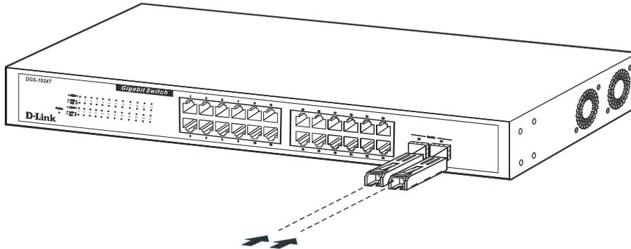
Figure 1- 5. Mini-GBIC modules plug-in to the Switch
