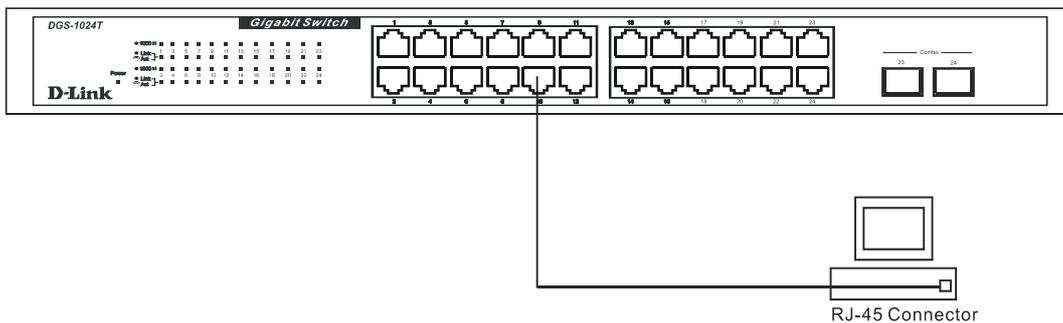
**Figure 2- 4. Switch connected to an end node**
