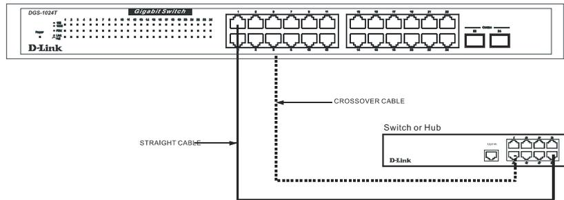
Figure 2- 5. Switch connected to a port on a hub or switch using either a straight or crossover cable—any standard Ethernet cable is fine
