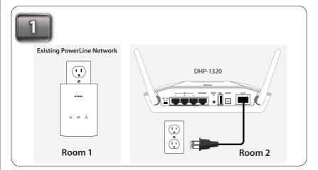
Plug one PowerLine AV adapter into an AC wall outlet. Verify that the Power LED is lit. If not, insert into another outlet. Now plug the DHP-1320 power chord into an AC wall outlet. Verify the Power LED is lit.
