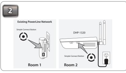
To secure your network, press the Simple Connect button for 2 seconds on one of the adapters. The Power LED will start to blink. Then, within 2 minutes, press the Simple Connect button on the DHP-1320 for 2 seconds.
