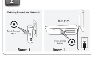
To secure your network, press the Simple Connect button for 2 seconds on the DHP-1320. The Power LED will start to blink. Then, within 2 minutes, press the Simple Connect button on the adapter for 2 seconds. Verify if the PowerLine AV LED is on.
