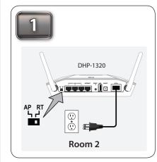
Place the DHP-1320 in a different area of your home. Next, move the switch to "AP". Connect the power cord into the power receptor. Then, plug into a wall outlet and turn on the device.
