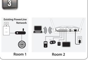
Connect one end of the Ethernet cable to the back of the DHP-1320 and attach the other end of the Ethernet cable to a PC, game console, NAS or TV.
