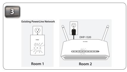
Verify that the PowerLine LED is lit on both the router and the adapter. This indicates that your PowerLine devices are properly connected to each other. If the PowerLine LED is not lit, connect the adapter(s) in different outlets and repeat Step 2.
