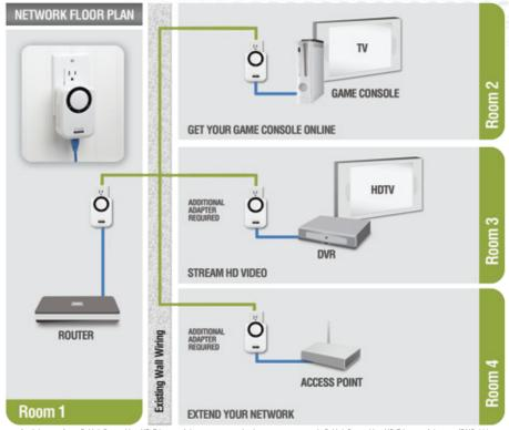
A minimum of two D-Link PowerLine HD Ethernet Adapters are required to create a network. D-Link PowerLine HD Ethernet Adapters (DHP-300, DHP-301) may coexist, but are not compatible or interoperable, with D-Link HomePlug AV Ethernet Adapters (DHP-304, DHP-305).
