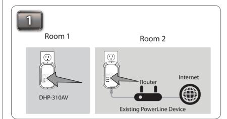
You must have at least one existing PowerLine device for the DHP-310AV to work. Plug the DHP-310AV into an AC wall outlet. Verify that the Power LED is lit. If not, insert into another outlet.
