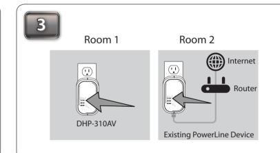
Once the Power LEDs stop blinking, verify that the PowerLine LED is lit on both adapters. This indicates that your adapters are properly connected to each other. If the LED is not lit, insert the DHP-310AV into a different outlet and repeat step 2.
