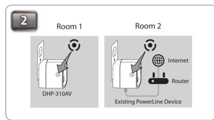
To secure your network, press the Simple Connect button for 2 seconds on one of your existing PowerLine devices. The Power LED will start to blink. Then, within 2 minutes, press the Simple Connect button on the DHP-310AV for 2 seconds.
