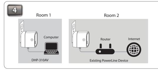
You may now attach Ethernet devices such as a computer, game console, or media player via an Ethernet cable. With the Ethernet device powered on, verify that the Ethernet LED is lit on the adapters to indicate a good connection. Setup is complete.
