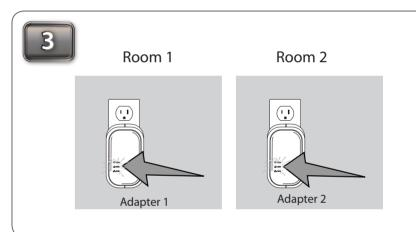
Once the Power LEDs stop blinking, verify that the PowerLine LED is lit on both adapters. This indicates that your adapters are properly connected to each other. If the LED is not lit, insert one or both adapters into different outlets and repeat step 2.
