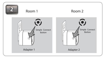
To secure your network, press the Simple Connect button for 2 seconds on one of the adapters. The Power LED will start to blink. Then, within 2 minutes, press the Simple Connect button on the other adapter for 2 seconds.
