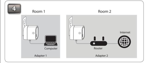
You may now attach Ethernet devices such as a router, computer, or game console via an Ethernet cable. With the Ethernet device powered on, verify that the Ethernet LED is lit on the adapters to indicate a good connection. Setup is complete.
