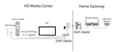
Note: A minimum of two D-Link PowerLine AV devices are required to create a PowerLine Network.
