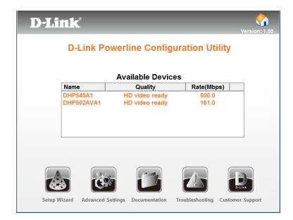
The setup wizard is designed to assist the installation of your PowerLine network. Click the Setup Wizard icon on the left corner of utility to start the installation process.
