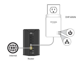
Plug in the other DHP-600AV adapter in the room that you want to extend your network. The Power LED will turn on.
