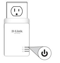
Verify that the PowerLine LEDs on both adapters are lit. If they are, the adapters are connected. If not, try another outlet.
