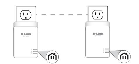
To secure your network, press the Simple Connect button (on the bottom) for two seconds on one of the adapters. The Power LED will start to blink. Then, within two minutes, press the Simple Connect button on the other adapter for two seconds. Once the Power LEDs stop blinking, verify that the PowerLine LED is lit on both adapters (as in Step 3). This indicates that your adapters are properly connected to each other.
