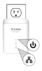
Werify that the PowerLine LEDs on both adapters are lit. If they are, the adapters are connected. If not, try another outlet.
