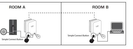
You can now connect another device using an Ethernet cable to the DHP-700AV adapter. Verify that the Ethernet LED is lit. Your installation is completed.
