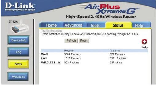
The screen above displays the Traffic Statistics. Here you can view the amount of packets that pass through the DI-624 on both the WAN and the LAN ports. The traffic counter will reset if the device is rebooted.
