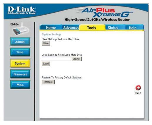
The current system settings can be saved as a file onto the local hard drive. The saved file or any other saved setting file can be loaded back on the Broadband Router. To reload a system settings file, click on **Browse** to browse the local hard drive and locate the system file to be used. You may also reset the Broadband Router back to factory settings by clicking on **Restore**.
