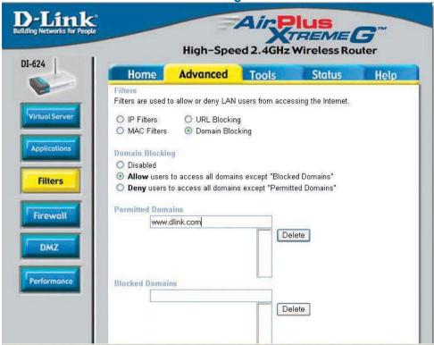
Domain Blocking is used to allow or deny LAN (Local Area Network) computers from accessing specific domains on the Internet. Domain blocking will deny all requests to a specific domain such as http and ftp. It can also allow computers to access specific sites and deny all other sites.
