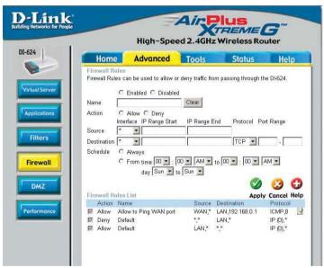
**Step 5** Select **LAN** as the **Destination** and enter the IP Address of the computer on your local network that you want to allow the incoming service to. This will not work with a range of IP Addresses.
