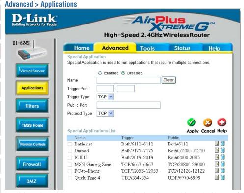
The DI-624S provides some predefined applications in the table on the bottom of the web page. Select the application you want to use and enable it.
