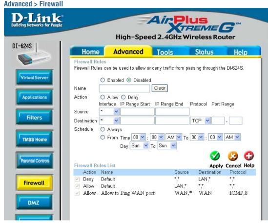
**Firewall Rules** is an advanced feature used to deny or allow traffic from passing through the DI-624S. It works in the same way as IP Filters with additional settings. You can create more detailed access rules for the DI-624S. When virtual services are created and enabled, it will also display in Firewall Rules. Firewall Rules contain all network firewall rules pertaining to IP (Internet Protocol).
