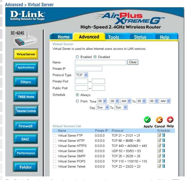
The DI-624S can be configured as a virtual server so that remote users accessing Web or FTP services via the public IP address can be automatically redirected to local servers in the LAN (Local Area Network).
