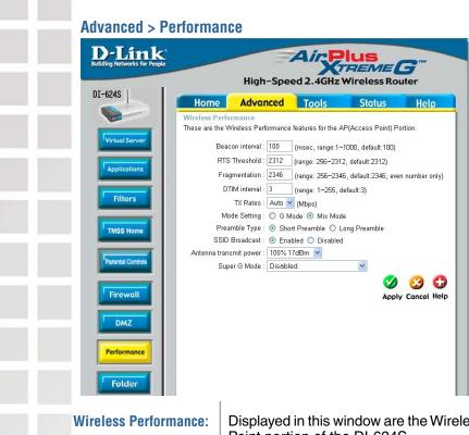
Displayed in this window are the Wireless Performance features for the Access Point portion of the DI-624S.
