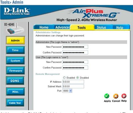
At this page, the DI-624S administrator can change the system password. There are two accounts that can access the Broadband Router's Web-Management interface. They are admin and user. Admin has read/write access while user has read-only access. User can only view the settings but cannot make any changes.
