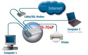
With the DI-704P you can share Internet access and resources such as printers in your home or office. Connect up to four computers and a printer with the DI-704P's parallel printer port.
