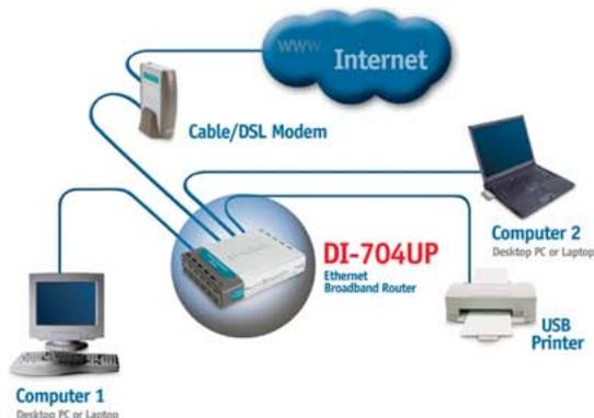
With the DI-704UP you can share Internet access and resources such as printers in your home or office. Connect up to four computers and a printer with the DI-704UP's USB printer port.
