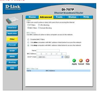
MAC (Media Access Control) Filters are used to deny or allow LAN (Local Area Network) computers from accessing the Internet and network by their MAC address.
