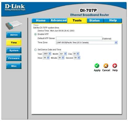
Set the time here by entering it manually or by using NTP (Network Time Protocol.) NTP is a standard protocol on the Internet that sychronizes the time settings accurately for all the computers on your network.
