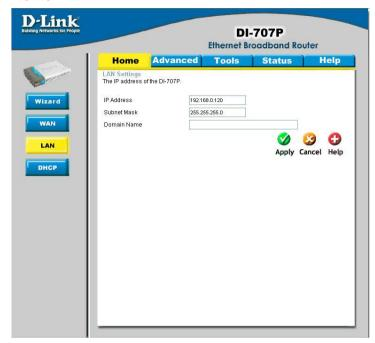
LAN is short for Local Area Network. This is considered your internal network. These are the IP settings of the LAN interface for the DI-707P. These settings may be referred to as Private settings. You may change the LAN IP address if needed. The LAN IP address is private to your internal network and cannot be seen on the Internet
