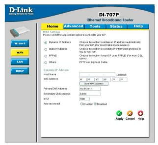
Most Cable modem users will select this option to obtain an IP Address automatically from their ISP (Internet Service Provider).
