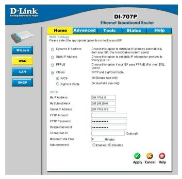
Point-to-Point Tunneling Protocol (PPTP) is a WAN connection used in Europe.
