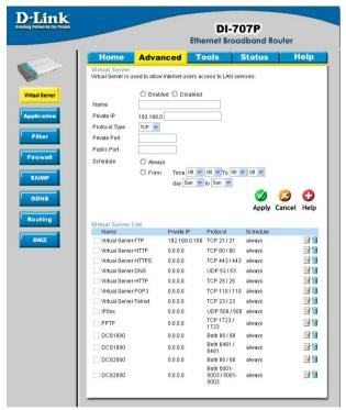
The DI-707P can be configured as a virtual server so that remote users accessing Web or FTP services via the public IP address can be automatically redirected to local servers in the LAN (Local Area Network).
