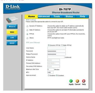
Most DSL users will select this option to obtain an IP address automatically from their ISP through the use of PPPoE.
