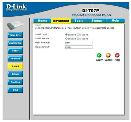
SNMP (Simple Network Management Protocol) is a widely used network monitoring and control protocol that reports activity on each network device to the administrator of the network. SNMP can be used to monitor traffic and statistics of the DI-707P. The DI-707P supports SNMP v1.
