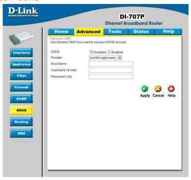
DDNS (Dynamic Domain Name System) keeps dynamic IP addresses (e.g., IP addresses assigned by a DHCP capable router or server) linked to a domain name. Users who have a Dynamic DNS account may use this feature on the DI-707P.
