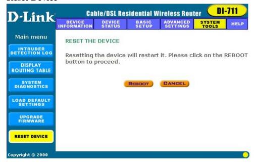
The Reset Device screen enables you to reboot the DI-711. If any changes are made and you want them to take effect, you will need to reset the DI-711 to do so. Click the "Reboot" button to reset the DI-711. Click the "Cancel" button to cancel.
