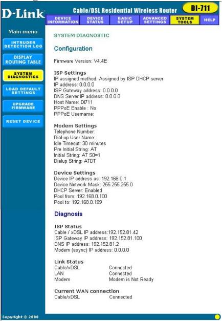
The System Diagnostics screen displays current status and connection information. This screen is similar to the Device Status screen, although both sections can be used to diagnose problems with your Internet connection.
