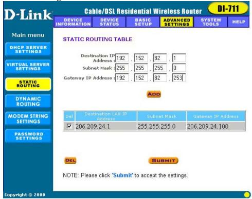
In Static Routing, the user has the ability to add a static route to the routing table by simple entering the destination IP, subnet mask, and gateway. Clicking on "Add" and then "Submit" which requires a restart for the IP address to be incorporated into the routing table.
