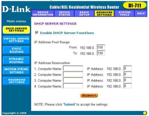
By default, the Wireless Broadband Router has DHCP server enabled to assign an IP address ranging from 192.168.0.100 to 192.168.0.199. In addition, the router is capable of reserving up to four IP addresses within the local network for mail, web, or ftp server.
