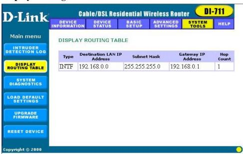
The Display Routing Table screen displays the routing table that the DI-711 is using. A router uses a routing table to keep track of what IP addresses there are and where the router should forward packets when it
