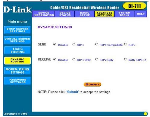
By default, the Wireless Broadband Router will not send or receive any routing Internet protocols (RIP) to update the routing table. However, the user can enable the Wireless Broadband Router to automatically send and receive RIP packets to establish routes for commonly used paths.
