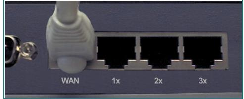
Finally, connect computers with ethernet adapters to one of the LAN ports on the DI-713P.
