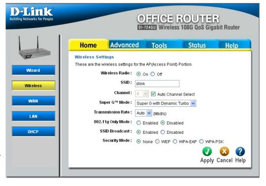
Super G<sup>™</sup> Mode: The default Super G setting is Super G with Dynamic Turbo. Super G is a group of performance enhancement features that increase end user application throughput in an 802.11g network. Super G is backward compatible to standard 802.11g devices. For top performance, all wireless devices on the network should be Super G capable. Select either Disabled, Super G without Turbo, Super G with Dynamic Turbo, or Super G with Static Turbo.
