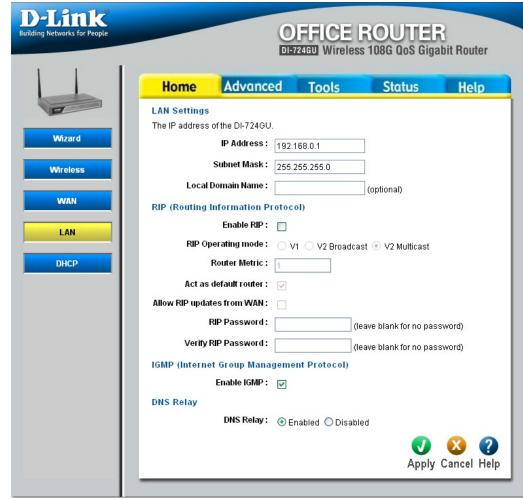
Router Metric: The additional cost of the routing a packet through this router. The normal value for a simple network is 1. This metric is added to routes learned from other routers; it is not added to static or system routes.
