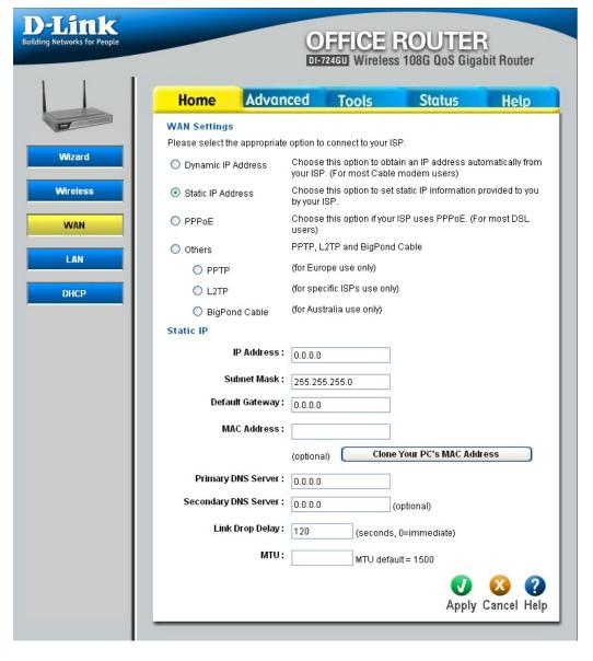
MAC Address You can either type in an alternate MAC address (for example, the MAC address of the router initially connected to the (continued): ISP) or copy the MAC address of a PC. To copy the MAC address of the computer that initially connected to the ISP, connect to the router using that computer and click the Clone Your PC's MAC Address button. The WAN port will then use the MAC address of the network adapter in your computer.
