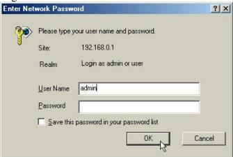
In order to configure the DI-804 you must input the user-name into the **User Name** box. Enter the password into the **Password** box and press the **OK** button. The default User Name is "admin". There is no default password, leave the Password field blank.
