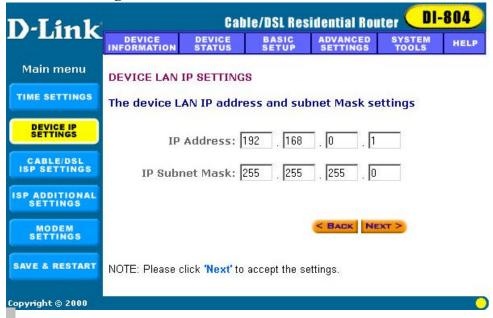
You have to give your Internet gateway an IP address on your "private" network. This is not the "public" IP address from your ISP but the local internal LAN IP address. The IP address of "192.168.0.1" is the default IP address of the LAN port in the broadband router.
