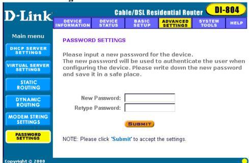
You can give your Internet gateway a new password. This password will be required the next time and subsequent times you configure your Internet gateway. To enter a password, type your password in the new password field and type it again in the retype password field.
