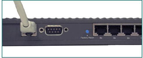
Finally, connect the computer to one of the LAN ports on the DI-804.
