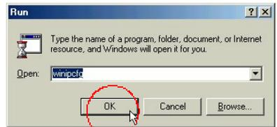
Click on the “**Release All**” and then on the “**Renew All**” button to obtain an IP address from the broadband router between 192.168.0.100. and 192.168.0.199.
