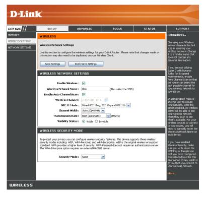
Visibility Status: Select Invisible if you do not want the SSID of your wireless network to be broadcast by the DIR-625. If Invisible is selected, the SSID of the DIR-625 will not be seen by Site Survey utilities so your wireless clients will have to know the SSID of your DIR-625 in order to connect to it.
