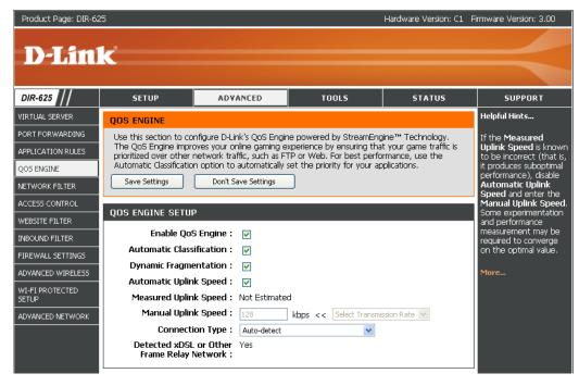
Manual Uplink The speed at which data can be transferred from the router to your ISP. This is determined by your ISP. ISPs often note speed Speed: as a download/upload pair. For example, 1.5Mbits/284Kbits. Using this example, you would enter 284. Alternatively you can test your uplink speed with a service such as www.dslreports.com.
