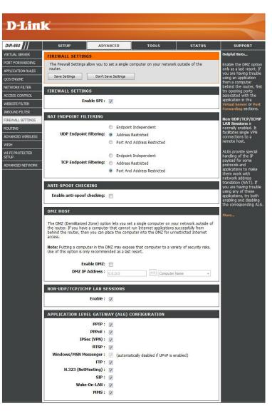
Non-UDP/TCP/ICMP Enable this feature to allow the router' NAT to track application that uses protocols other than UDP, TCP or ICMP. LAN Sessions:
