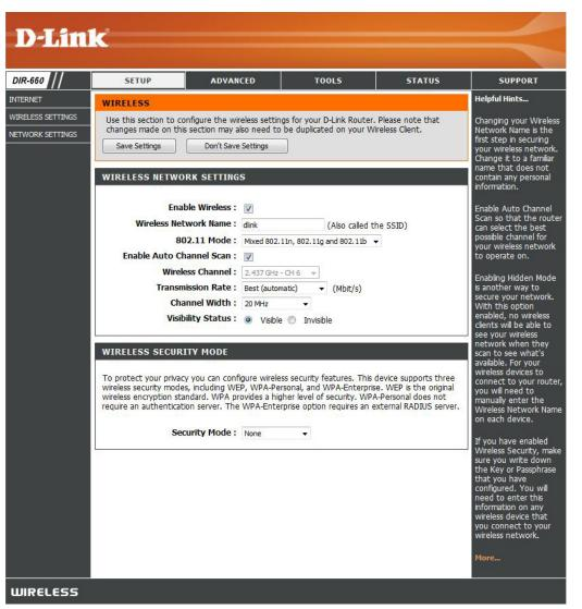
Mixed 802.11n, 802.11b, and 802.11g - Select if you are using a mix of 802.11n, 11g, and 11b wireless clients. Mixed 802.11n and 802.11g - Select if you are using a mix of 802.11n and 802.11g wireless clients.
